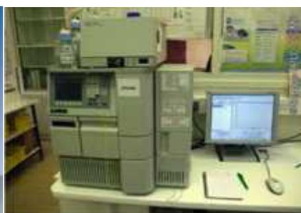
Figure XXIV: HPLC (WATERS 298 PHOTODIODE ARRAY DETECTORS)
