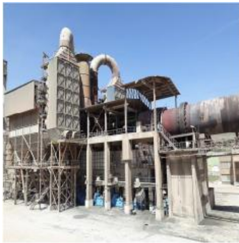
Figure 4.1-b. Cooler system with its heat exchanger and filter to the left and kiln end appears to right.
