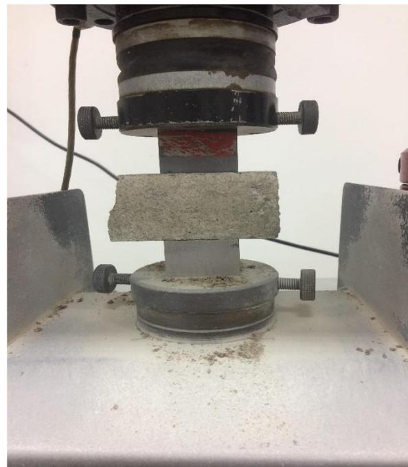
*Figure III.23(b)-Essai de compression.*
