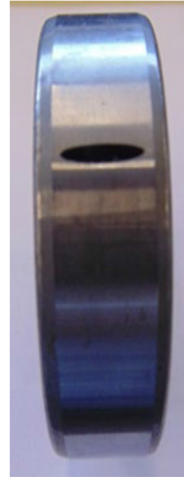
Fig. 8. Image of a defect on the ball bearing.
