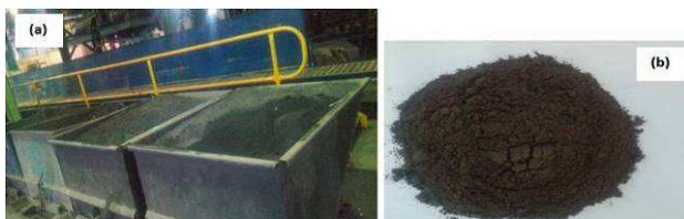
Figure 1. Foundry sand wastes used in this work (a) rejected zone (b) FWS as sand
