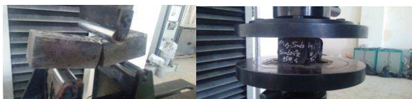
Figure 6. Mechanical tests (compressive and flexural strength)
