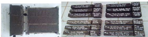
Figure 5. Prismatic (40x40x160 mm 3 ) and cubic (50x50x50 mm 3 ) samples of mortars
