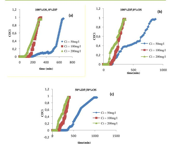
*Figure 6:* Breakthrough curves for adsorption of MB by olive stone (a); date pit (b); mixture of date pit and olive stone (c) for different concentration values (pH = 5.6 H = 5 cm Q = 8.15 ml / min)
