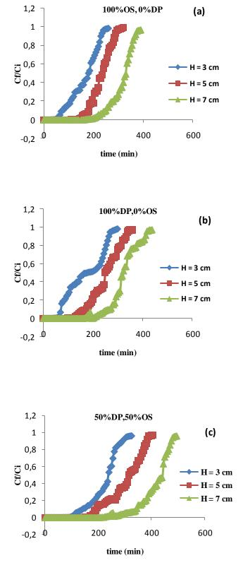
**Figure 4:** Breakthrough curves for adsorption of *MB* by olive stone (*a*); date pit (*b*); mixture of date pit and olive stone (*c*) for different bed height values (pH = 5.6 Q = 8.15 ml / min Ci = 100 mg / l)
