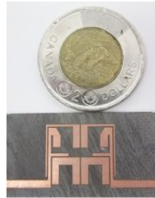
Figure 7. The photograph of the fabricated filter
