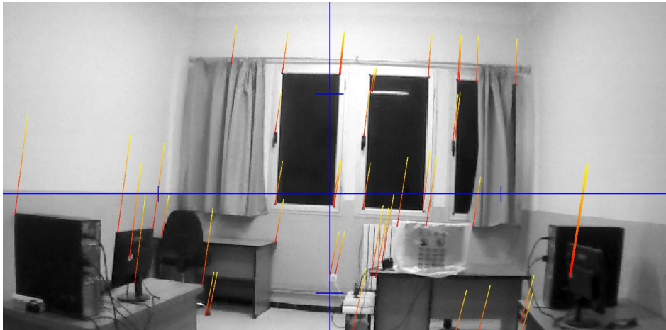
Figure 3-3: Initialization procedure of PTAM. Every line corresponds to a successfully tracked keypoint.
