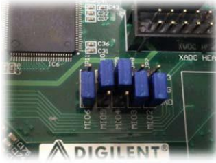
Figure 3. 3: Jumper Settings to boot from SD Card
