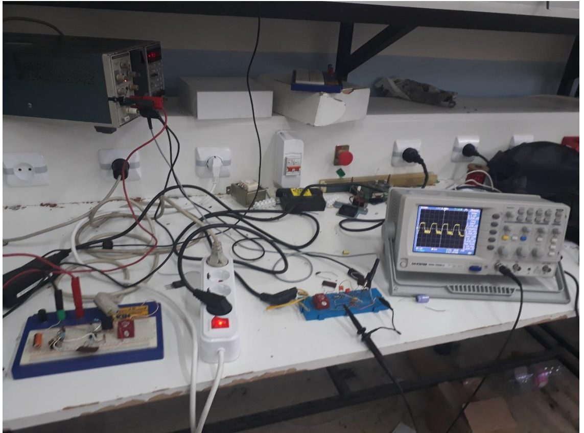
Figure 4.20 The Power Line Communication at Work.
