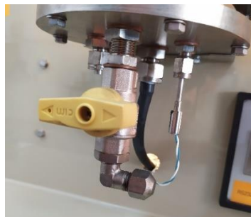
Figure 3.10 – La soupape de charge
