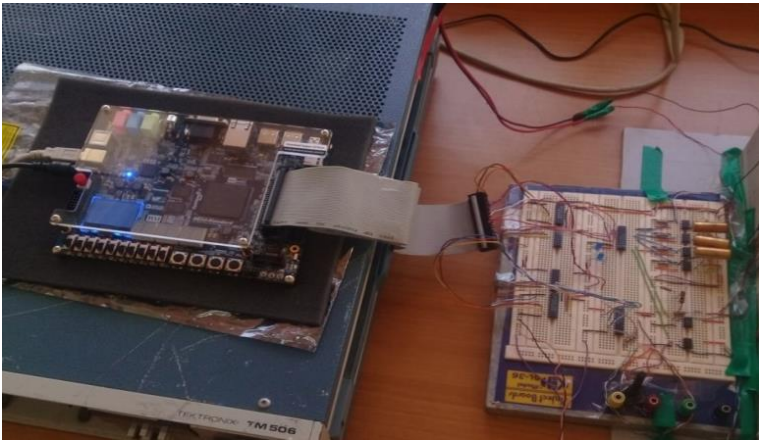
Figure 2.2 The Fpga connected to the off-ship system through a ribbon cable
