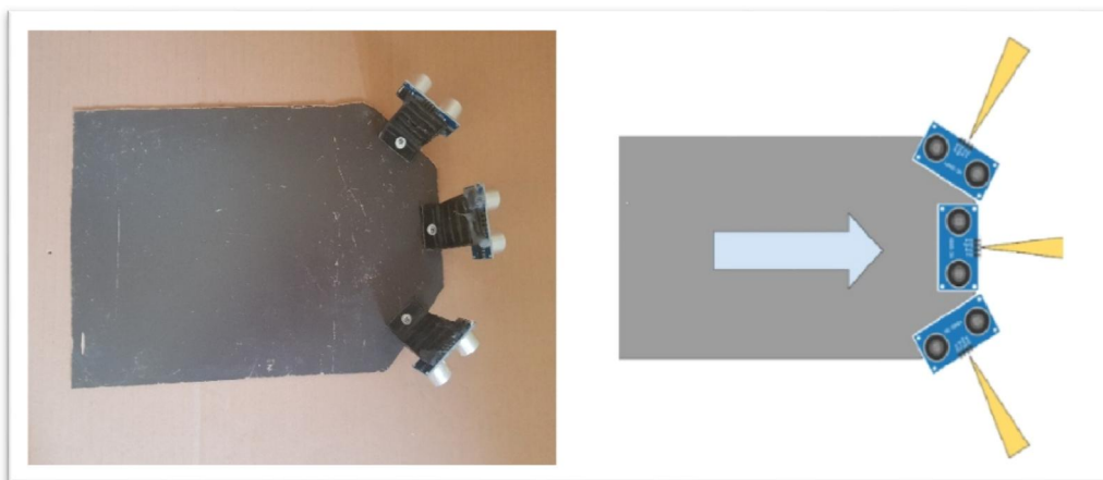
Figure 2.9. RC Car's ultrasound sensor placement.
