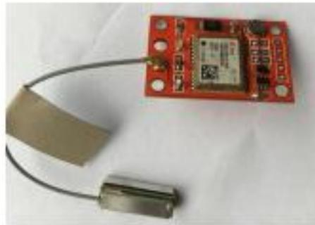
GY-NEO6MV2 board features the u-blox NEO-6M GPS module with antenna and built-in EEPROM. This is compatible with various flight controller boards designed to work with a GPS module.
