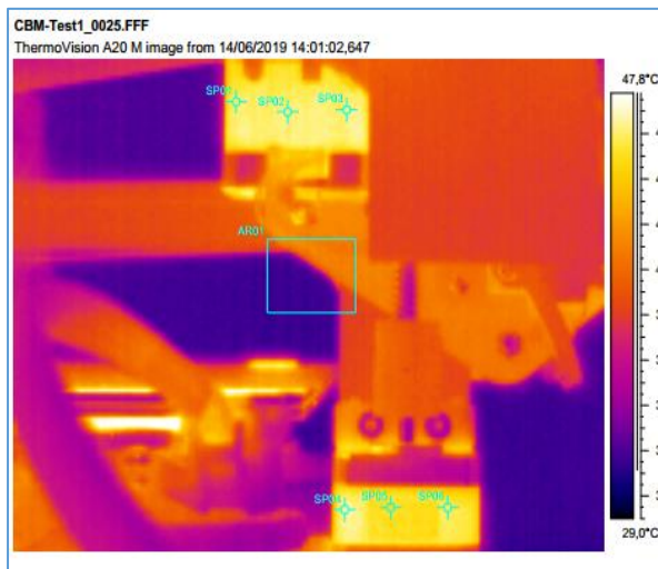
Fig. 47. Temperature field distribution at min 62:02, when SP01 from the M 1 reached the maximum temperature of 46.067°C
