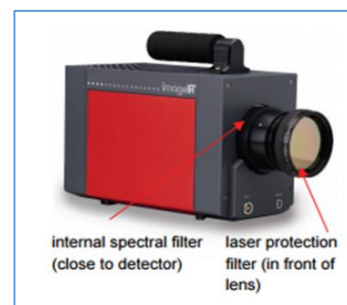
Fig. 25. Camera Image IR® series with motorized filter wheel [32]
