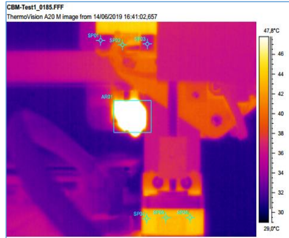
Fig. 64. Temperature field distribution in the nozzle area AR1 when maximum temperature was reached
