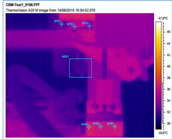
Fig. 50. Temperature field distribution at min 235:02, when SP02 from the M_1 reached the minimum temperature of 32.373°C
