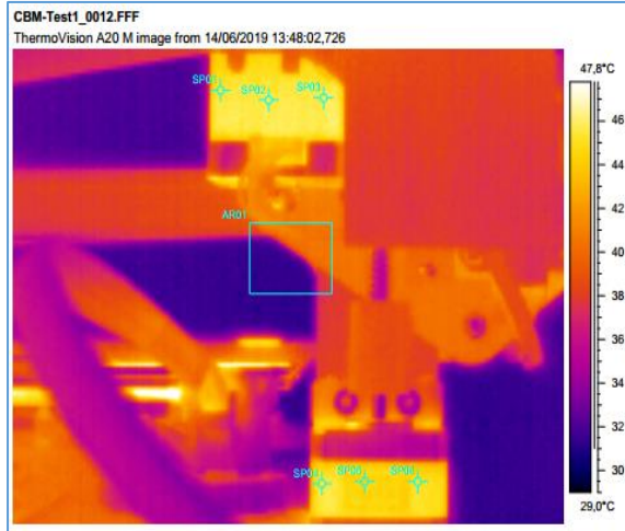
Fig. 49. Temperature field distribution at min 49:02 min, when SP02 from the M_1 reached the maximum temperature of 44.165°C
