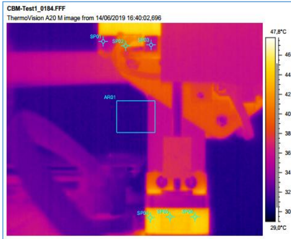
Fig. 63. Temperature field distribution in the nozzle area AR1 when maximum temperature was reached
