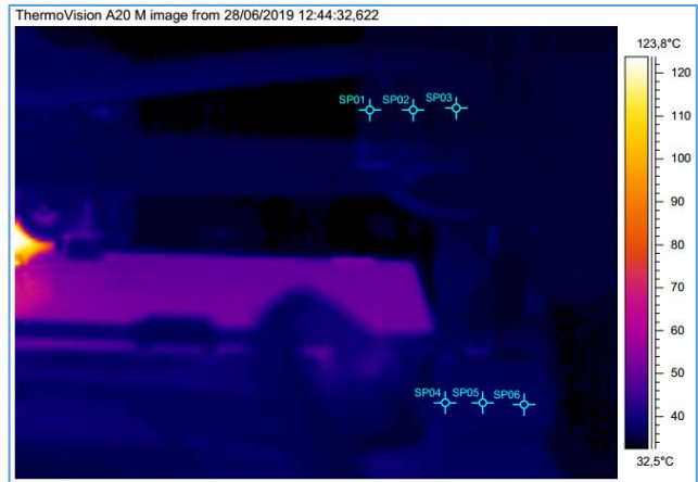
Fig. 83. Temperature field distribution at min 45:32, when SP06 from the M02 reached the minimum temperature of 34.558°C
