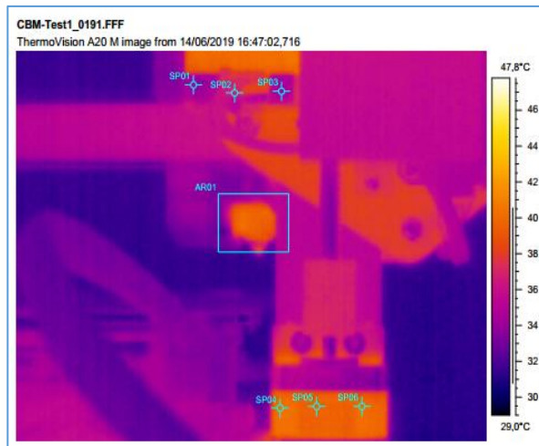
Fig. 66. Temperature field distribution in the nozzle area AR1 when maximum temperature was reached
