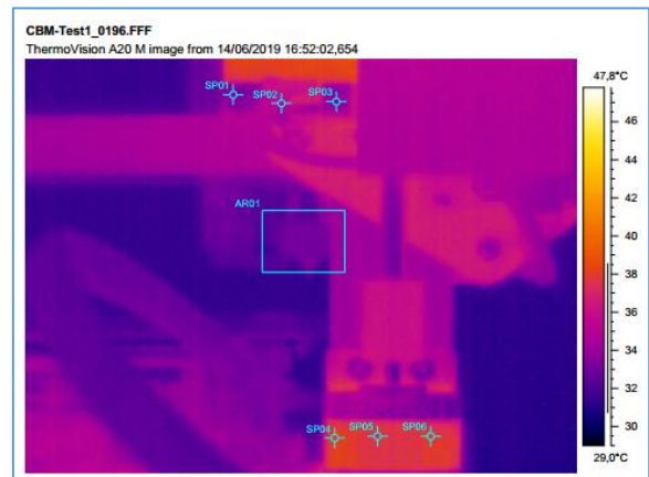
Fig. 60. Temperature field distribution at min 233:02 during the cooling phase
