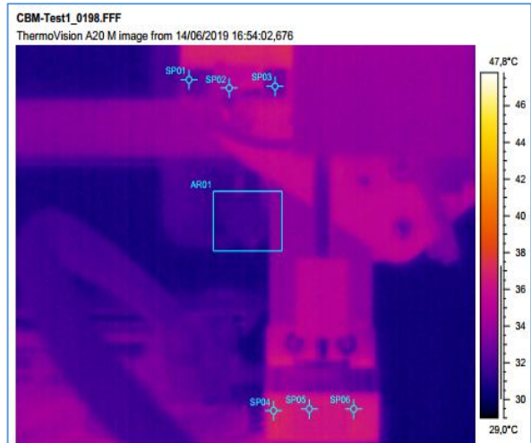
Fig. 58. Temperature field distribution at min 235:02, when SP06 from the M 2 reached the minimum temperature of 34.336°C
