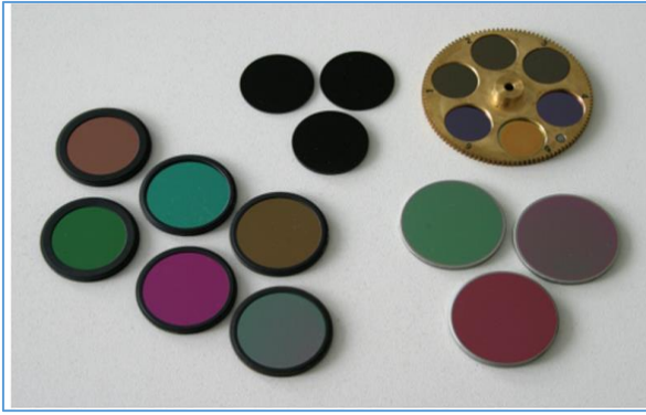
Fig. 20. Spectral filters for thermographic cameras
