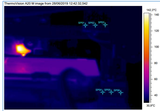
Fig. 77. Temperature field distribution at min 43:32, when SP03 from the M01 reached the minimum temperature of 32.689°C
