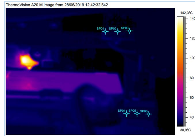
Fig.75. Temperature field distribution at min 43:32, when SP02 from the M01 reached the minimum temperature of 32.579°C
