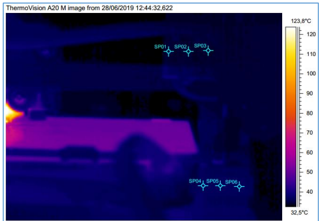
Fig. 79. Temperature field distribution at min 45:32, when SP04 from the M02 reached the minimum temperature of 34.836°C
