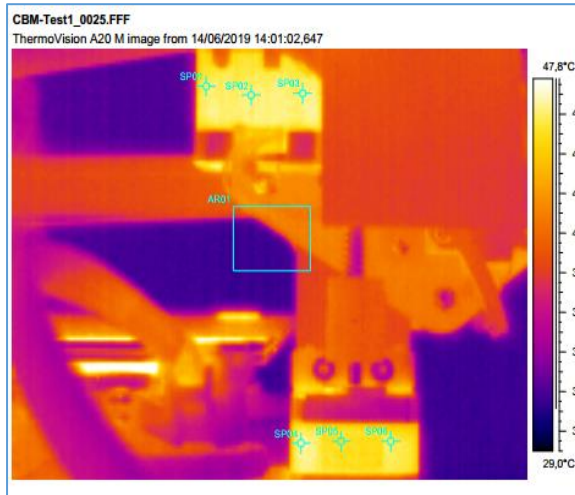
Fig. 57. Temperature field distribution at min 62:02, when SP06 from the M 2 reached the maximum temperature of 44.109°C
