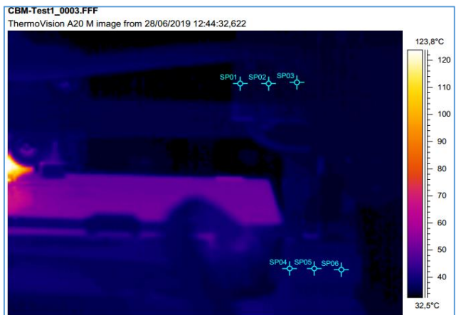
Fig. 81. Temperature field distribution at min 45:32, when SP05 from the M02 reached the minimum temperature of 34.543°C
