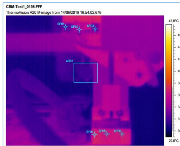
Fig. 48. Temperature field distribution at min 235:02, when SP01 from the M 1 reached the minimum temperature of 32.641°C
