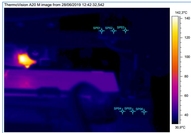
Fig. 73. Temperature field distribution at min 43:32, when SP01 from the M01 reached the minimum temperature of 32.516°C
