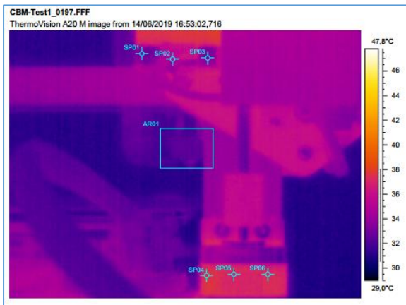
Fig. 59. Temperature field distribution at min 222:02 during the cooling phase
