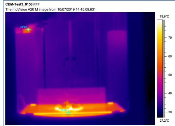
Fig. 100. Glass plate temperature of 69.282°C, during the cooling phase, at time 166:09 min
