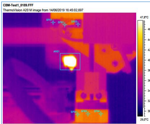
Fig. 65. Temperature field distribution in the nozzle area AR1 when maximum temperature was reached
