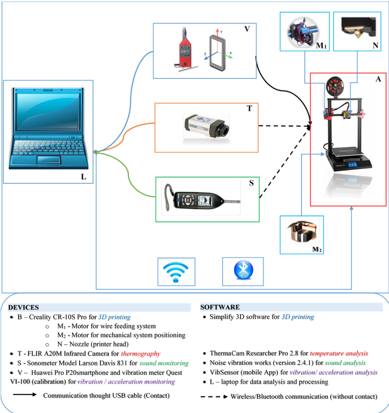
Fig. 70. The setup of the experimental Test 2. Schematic diagram
