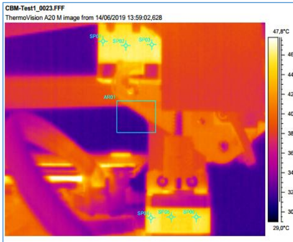
Fig. 51. Temperature field distribution at min 60:02, when SP03 from the M_1 reached the maximum temperature of 44.444°C
