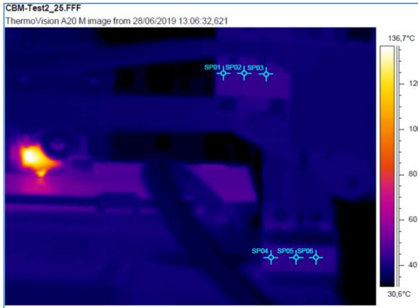
Fig. 82. Temperature field distribution at min 77.32, when SP06 from the M02 reached the maximum temperature of 45.352°C
