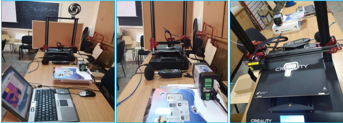
Fig. 45. 3D printing process monitoring using thermography. Experimental test 1
