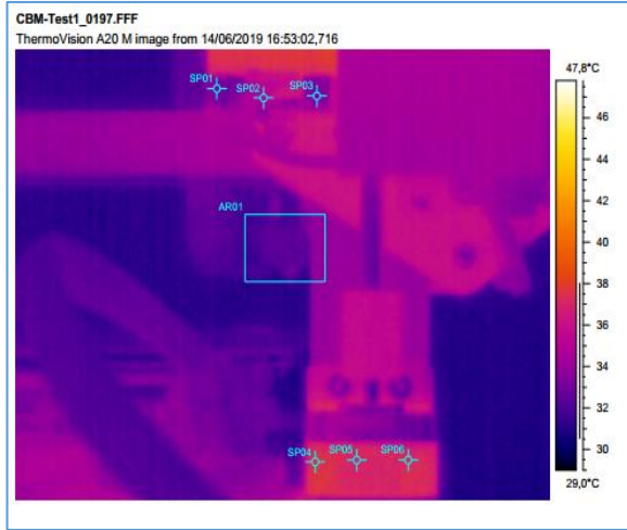
Fig. 61. Temperature field distribution at min 234.02, during the cooling phase
