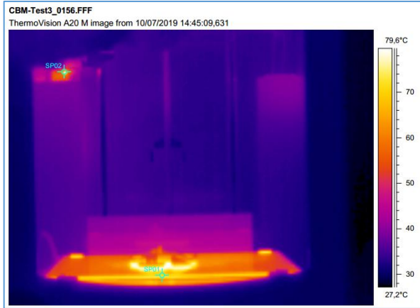
Fig. 99. Nozzle temperature of 59.321°C, during the cooling phase, at time 166:09 min
