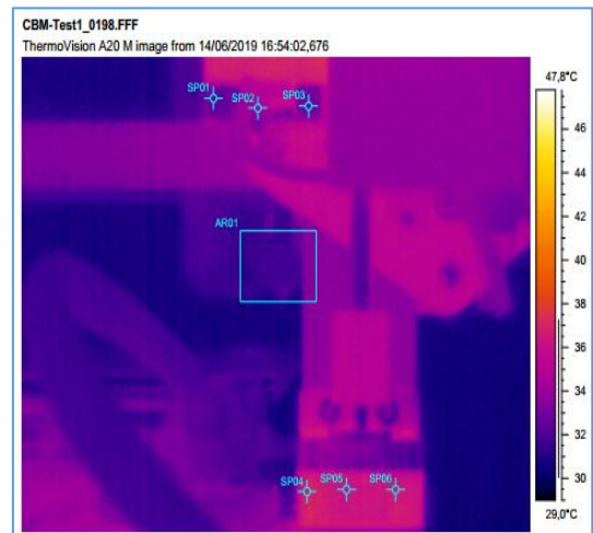
Fig. 54. Temperature field distribution at min 235:02, when SP04 from the M_2 reached the minimum temperature of 34.640°C
