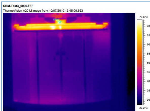
Fig. 97. Nozzle temperature of 70.345°C, during the 3D printing process, at time 106:09min
