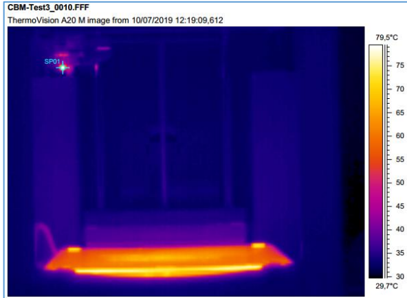
Fig. 93. Nozzle temperature of 61.235°C, before starting the 3D printing process, at time 20:09 min
