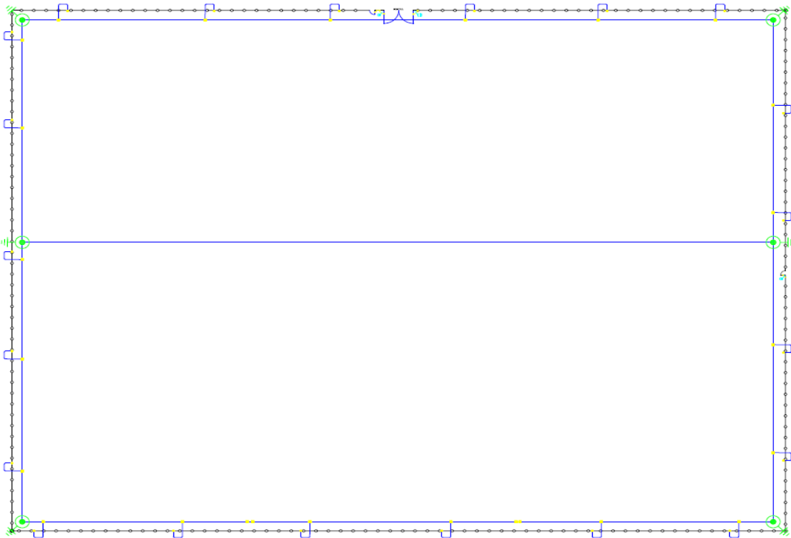
Figure IV. 3: earthing loop layout
