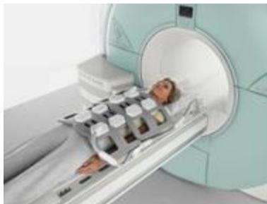
**Figure I.11 :** Antennes surfaciques
