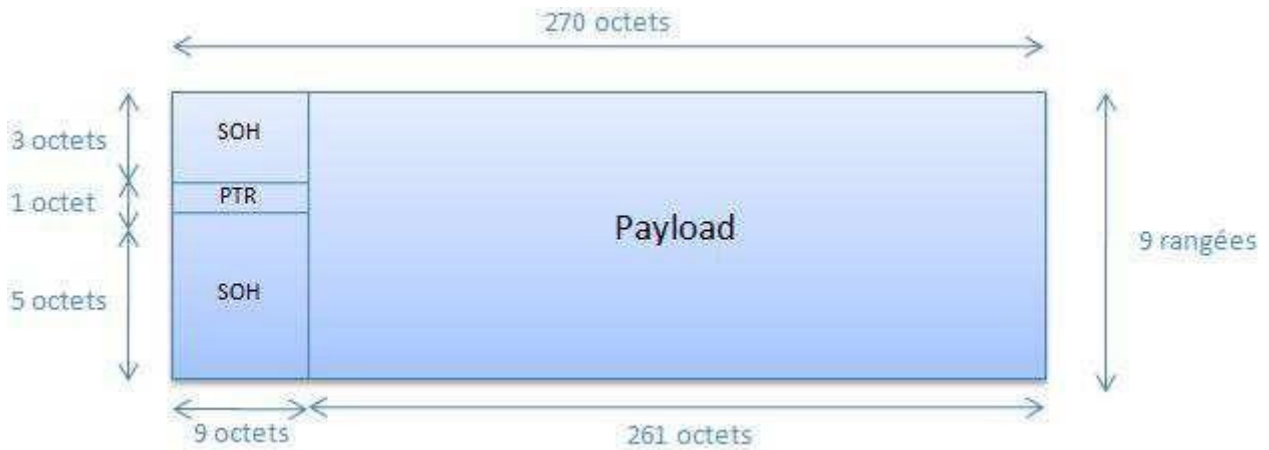
Figure 3.2: Structure de la trame SDH STM-1
