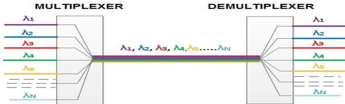
Figure 2-17: Technique de multiplexage
