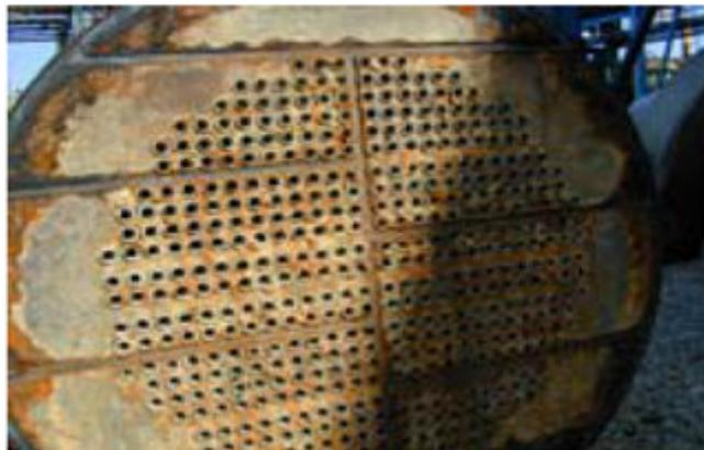
**Figure (3.6) :** Important corrosion.
