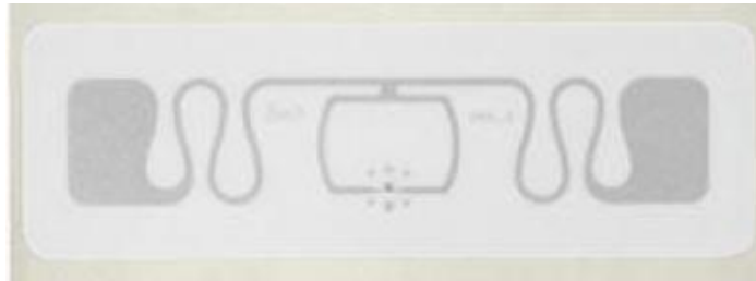
Figure 2.5: Passive RFID tag [14]
