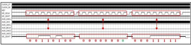
Figure 3.4: Transmission of Register 1 Data Configuration
