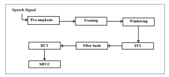
Figure 1.2: MFCC Block Diagram
