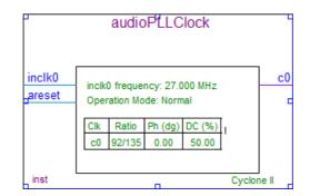
Figure 2.9: clock divider block
