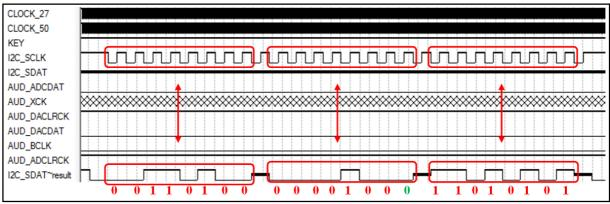
Figure 3.6: Transmission of Register 4 Data Configuration
