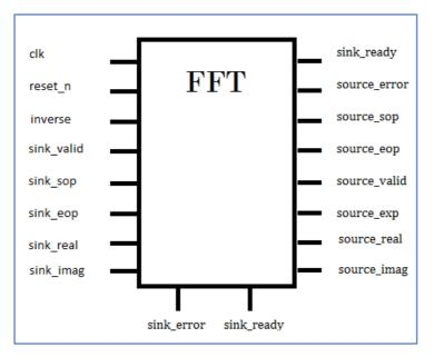
Figure 1.8: FFT IP core I/O
