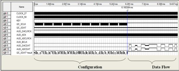
Figure 3.1: Audio Codec Simulation
