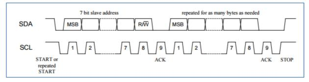
**Figure 1.7:** Data Transmission in the I<sup>2</sup>C Bus [23].
