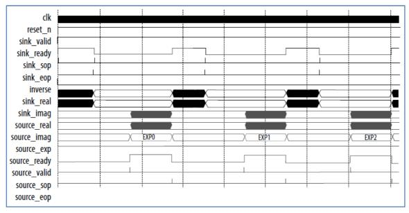
Figure 2.14: FFT Burst Data Flow Simulation Waveform [2]
