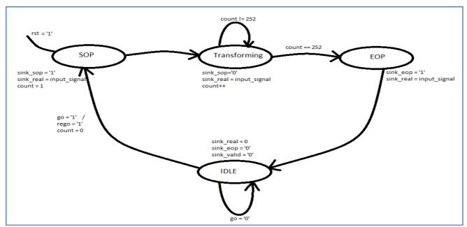
Figure 2.15: FFT Module FSM Diagram
