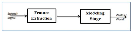
Figure 1.1: Block Diagram of Speech Recognition
