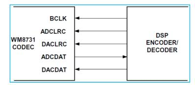
Figure 2.6: Slave Mode Connections [20]
