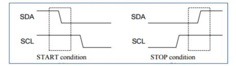
Figure 1.6: Start and Stop Condition of I<sup>2</sup>C Bus [23].
