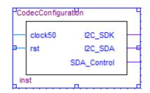
Figure 2.4: Audio codec controller block
