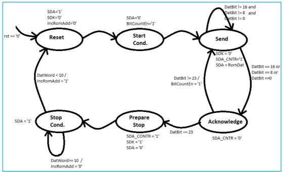
Figure 2.3: I2C FSM diagram
