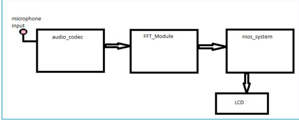
Figure 2.1: General implementation block diagram
