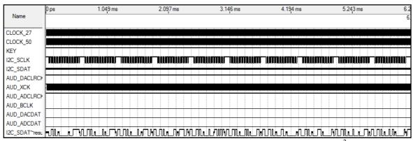
Figure 3.2: Transmission of Ten Frames of Data to the Wolfson Chip Using I<sup>2</sup>C Protocol
