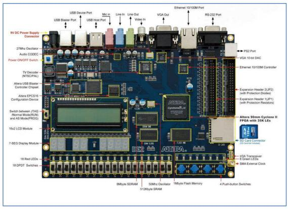
Figure 1.4: DE2 Board Top View [8].
