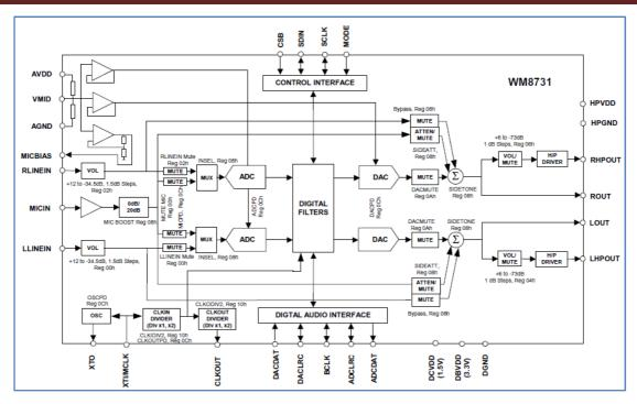
Figure 1.5: Functional Block Diagram of WM8731 Audio CODEC [20].
