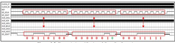
Figure 3.5: Transmission of Register 2 Data Configuration
