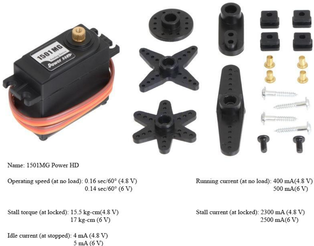
Fig 2.7: Power HD 1501 parts and specs [7].
