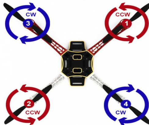
Figure 2.1: Quad-rotor in X configuration.
