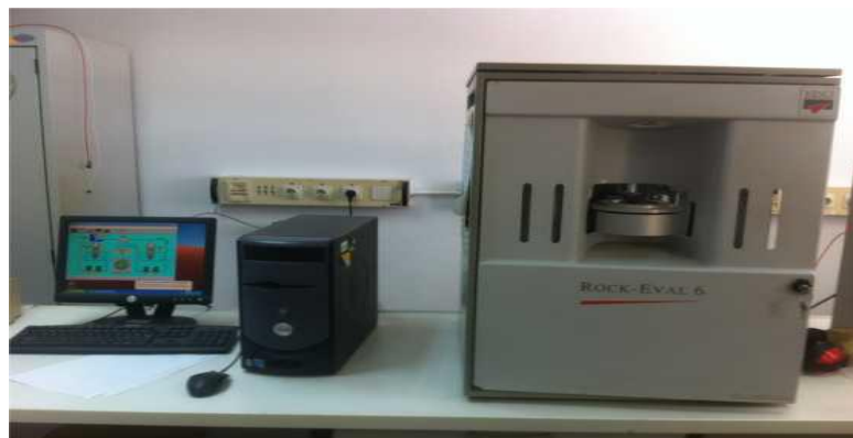
Figure III.1. Appareillage de pyrolyse Rock- Eval 6 [14]
