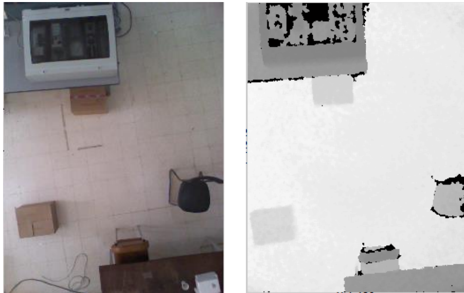
Fig 4-3. RGB and depth images acquired by the second Kinect.
