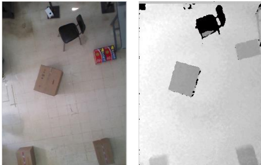
Fig 4-2. RGB and depth images acquired by the first Kinect.
