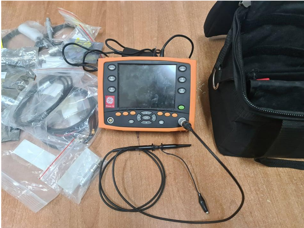
Fig VI.2 Eddy current fault-finding apparatus
