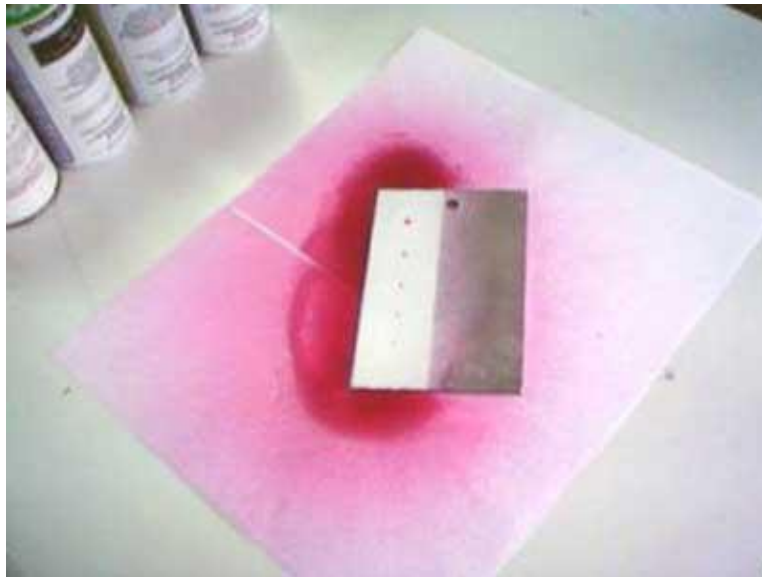
Step 6: After a pause, the image of the defects appears on the surface.
