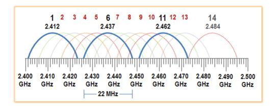
FIGURE 2.7 – Channels and interference on a WiFi network
