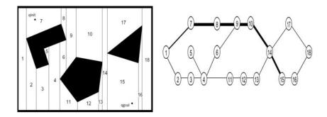
FIGURE 1.6 - Exact Cell Decomposition
