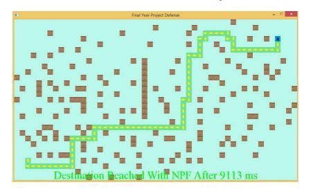
FIGURE 3.14 – Potential Field Implementation-Diagonals Are Not Allowed
