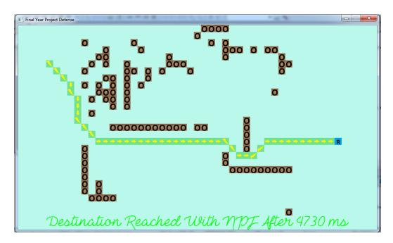
FIGURE 4.11 – Desired path produced using Numerical Potential Field
