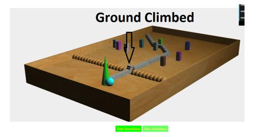
FIGURE 3.18 – Picture From Our 3D Simulator Uneven-terrain (ground climbed using Numerical Potential Field)
