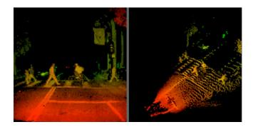
FIGURE 2.4 – In the image above, on the left is a LADAR image from the front of a vehicle stopped at a crosswalk in Santa Barbara, CA. On the right is the same LADAR data « viewed »from an overhead location highlights the 3-D nature of the data collected.
