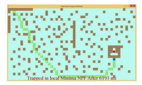
FIGURE 3.19 – Local Minima Detection Using Time Based Estimation
