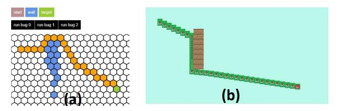
FIGURE 1.19 – bug0 implementation comparison (a)-Simulator from internet(no straight line) (b)-Illustration of our approach
