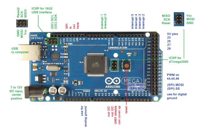
FIGURE 17 – Arduino Mega 2560
