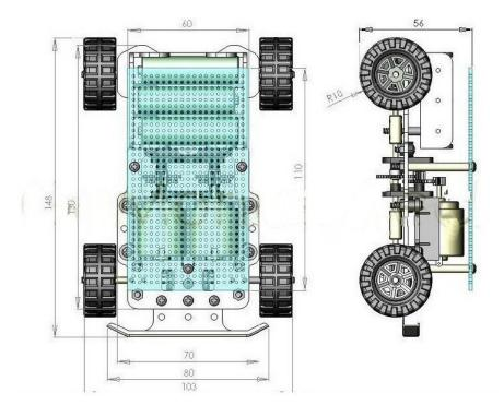
FIGURE 2.1 – Mobile Robot Platform Description (unit : mm)
