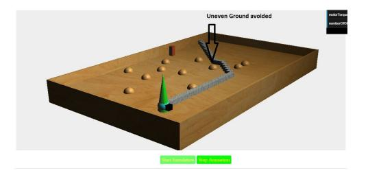
FIGURE 3.17 – Picture From Our 3D Simulator Uneven-terrain (ground circumvented using Numerical Potential Field)
