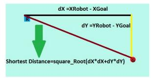
FIGURE 3.5 – Euclidean Shortest Distance in 2D Space(picture from our simulator)
