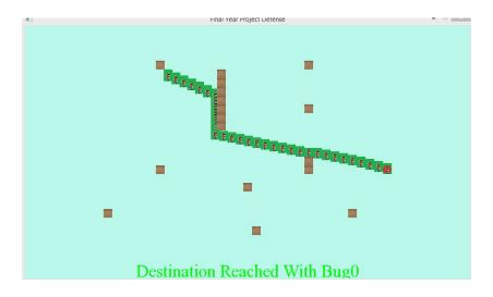
FIGURE 3.7 – Bug0 With Robot Position Discretization
