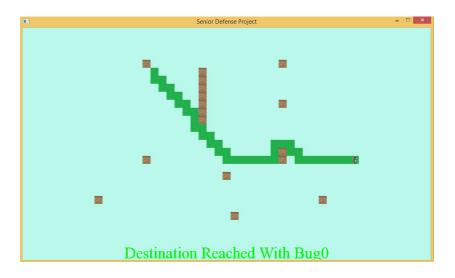
FIGURE 3.6 – Bug0 With Displacement Rounding
