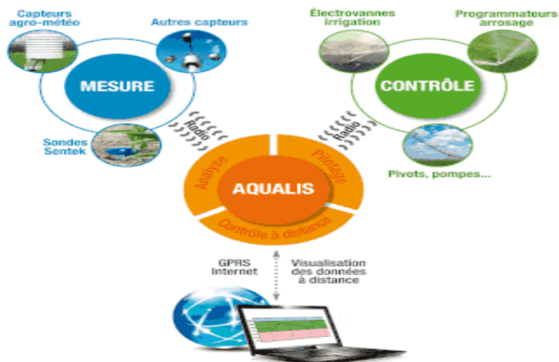
Figure II.9 : Principe de station Aqualis [12]
