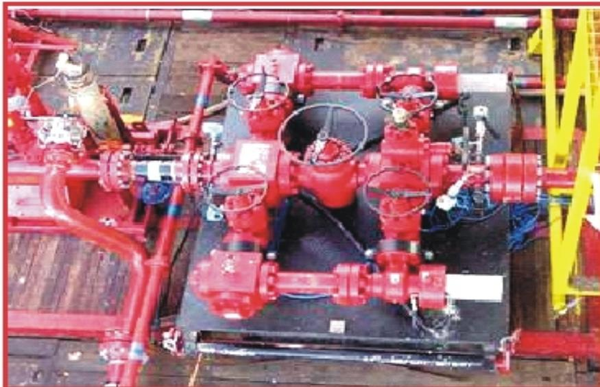
Figure 25 : Choke Manifold type 5000 psi.
