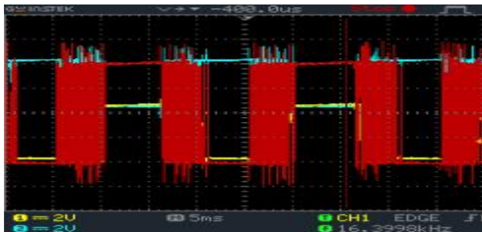
Figure 5.20 Inverter's output voltage (before filtering)
