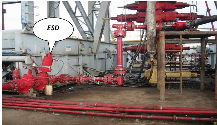
Figure 27 : Flow line secondaire.
