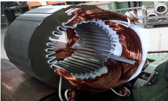
**Figure I.12.** Isolation des encoches statorique
