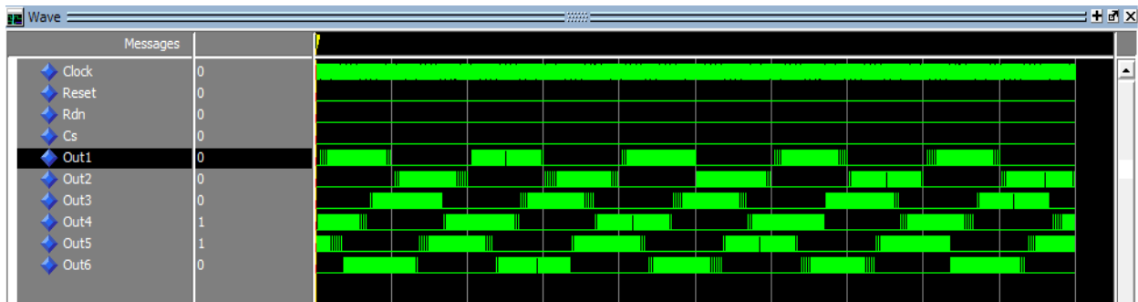
Figure 3-6 generation of the PWM pulses
