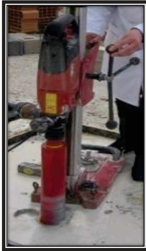
Figure 51 : Essai de carottage.
