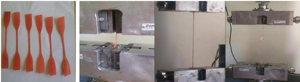
*Fig.V.5. Echantillon 1 (mélange [PEHD/PP/PET/Bentonite])*
