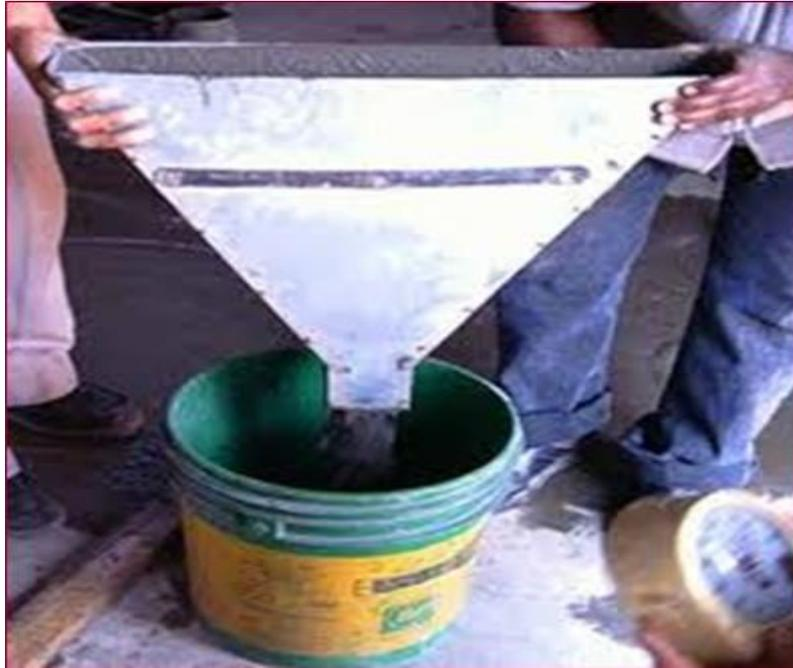
Figure III-2 : essai de V-funnel
