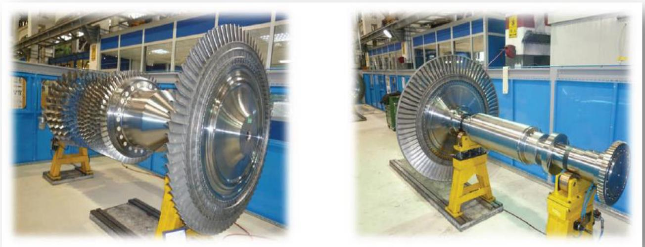
Figure 7: rotor HP; rotor BP
