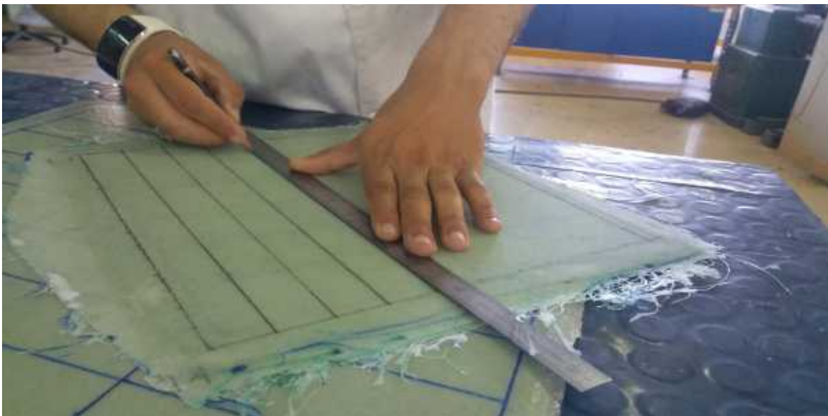
Figure .3.6 simple specimens made of glass /epoxy after preparation
