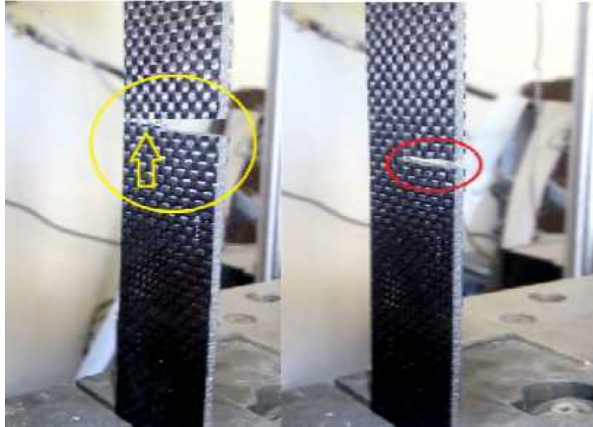
Figure .3.5 the specimen carbon /epoxy between the two jaws of the machine
