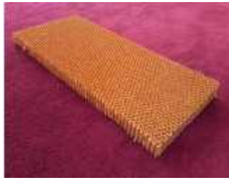
b) Aramide paper (Nomex) honeycomb core
