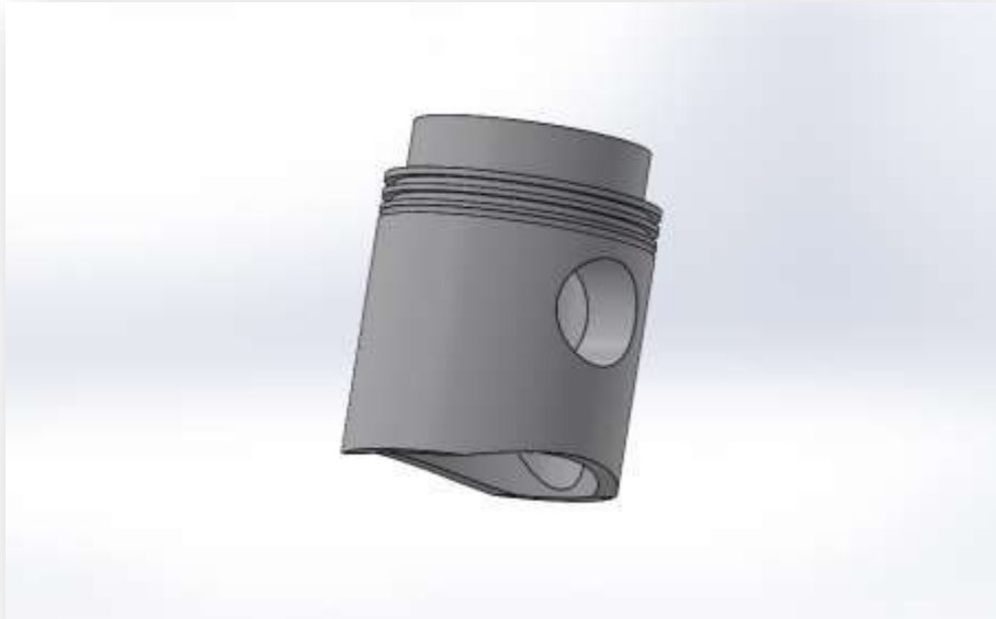
Figure 3.4: The piston skirt
