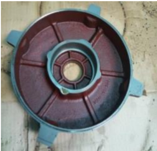
Figure I. 15. Flasque AS usiné
