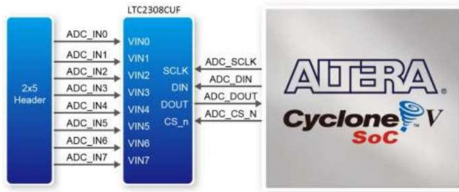
. Figure 3.2: Connections between the FPGA, 2x5 header, and the A/D converter [19]
