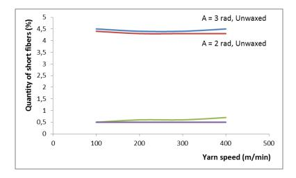
Fig.8. Quantity of short fibers at different angles, waxed and unwaxed yarns, (input tension 10 cN, needle gauge 14)
