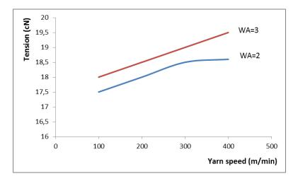
**Fig.5.** Variation of output tension at different yarn wrap angle (input tension = 10 cN, needle gauge 14)
