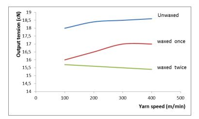
**Fig.6.** Variation of output tension with different yarn conditions (input tension 10 cN, needle gauge 14, A 3 radian)
