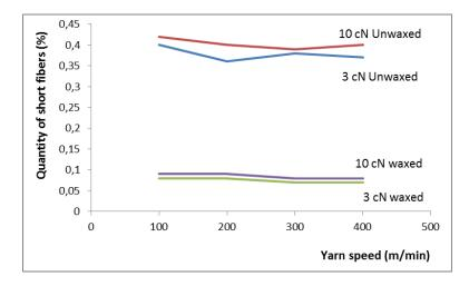
Fig.7. Amount of short fibers generated with different tensions, waxed and unwaxed yarns,
