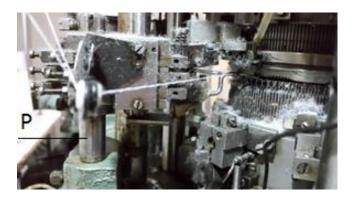
Fig.2. Short fibers in cotton deposited on circular knitting machine devices. Photo, Ali Bey H, Algiers
