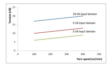
Fig.4. Variation of output tension with different input tension and speed (needle gauge 14, A = 3 radian)
