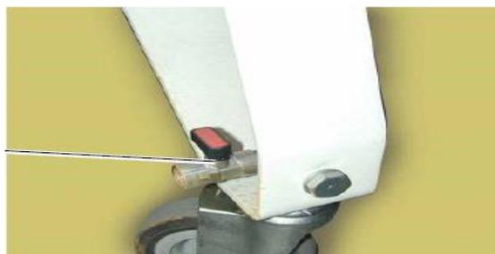
**Figure V.6:** Robinet Purger la condensation
