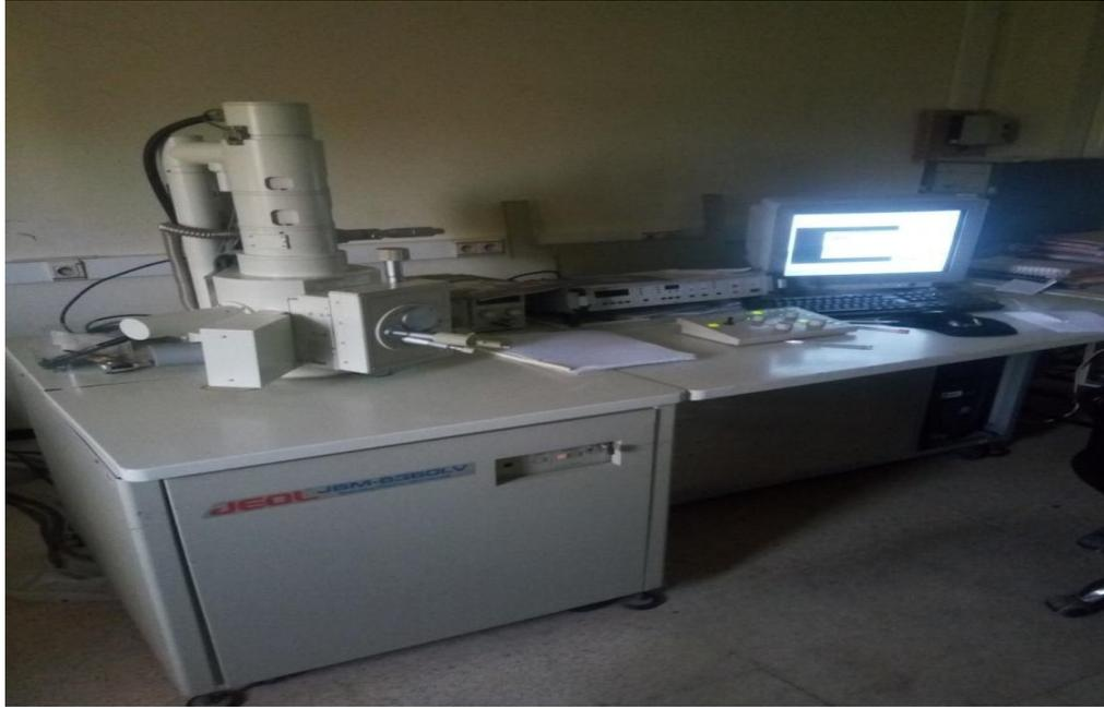
**Figure III.9:** Microscope (JEOL/JSM-6360LV).
